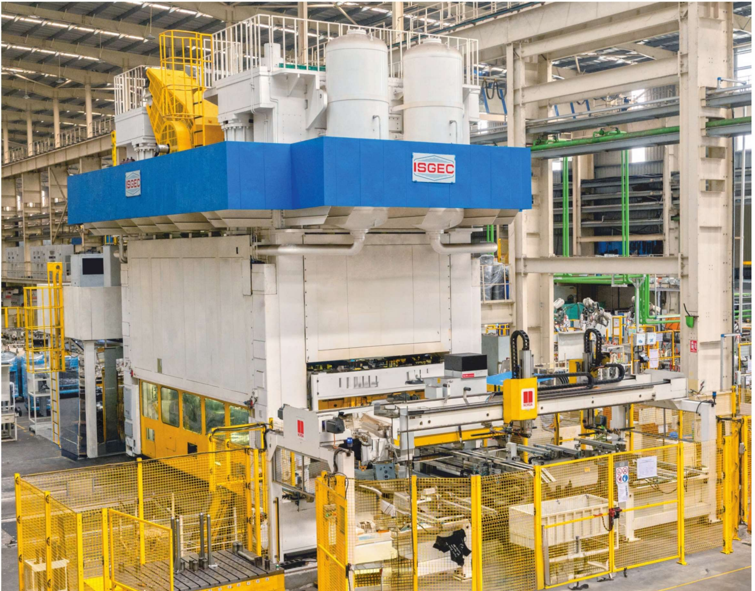
2500 T Link Drive Transfer Press (Bolster Size 6100 x 2500 mm) installed with a Tier-1 stamping supplier to Japanese OEM
