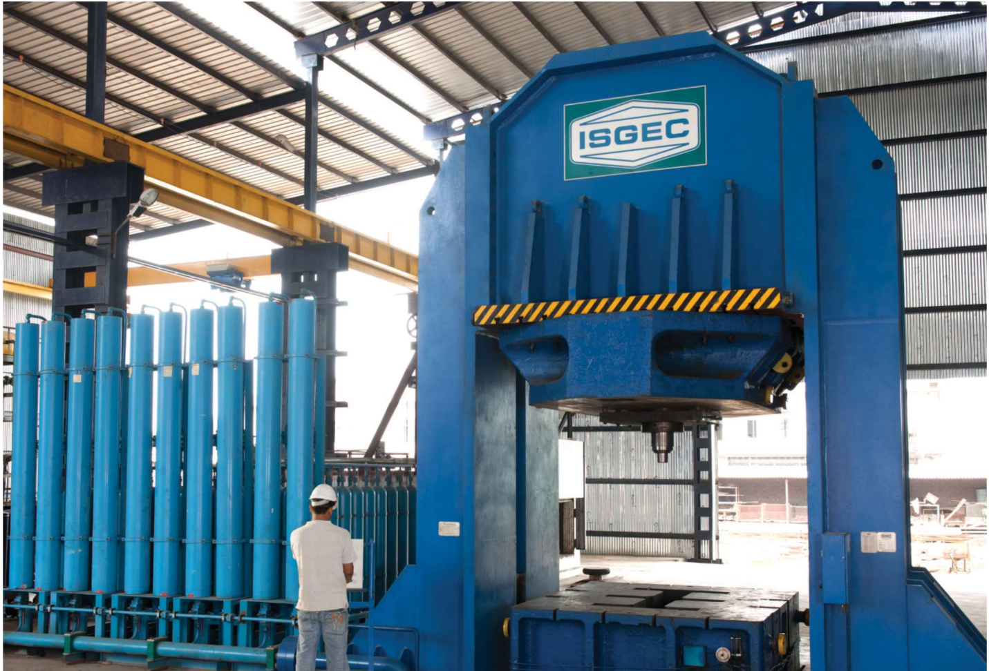
12500T Hydraulic Press with large Accumulator Bank is being used for Hot & Cold Forming of High Tensile Steel Plates for Defense & Aerospace Applications
