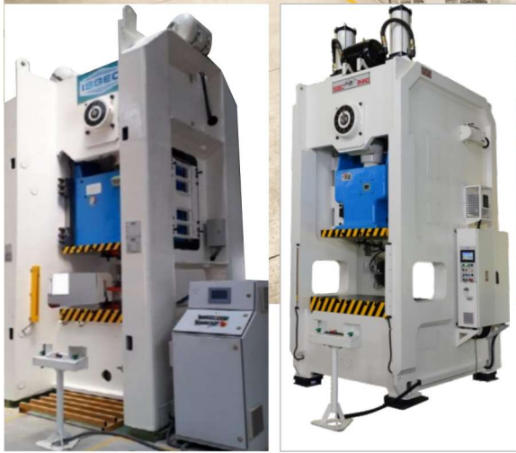
250 T MAX 1 Monolithic Frame Single Crank Press supplied to Auto Tier-2 in India. MAX 1 Models are available from 200 T to 400 T
