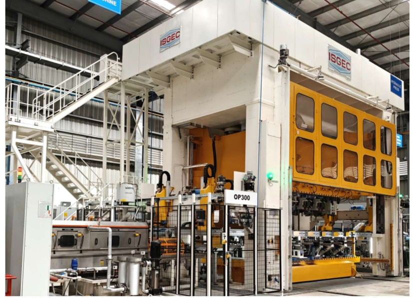
1200T High-Speed Hydraulic Transfer Press Line installed for a German MNC at their India plant. Equipped with a 6100 x 2500 mm bolster and a 3-axis electronic servo transfer system.
