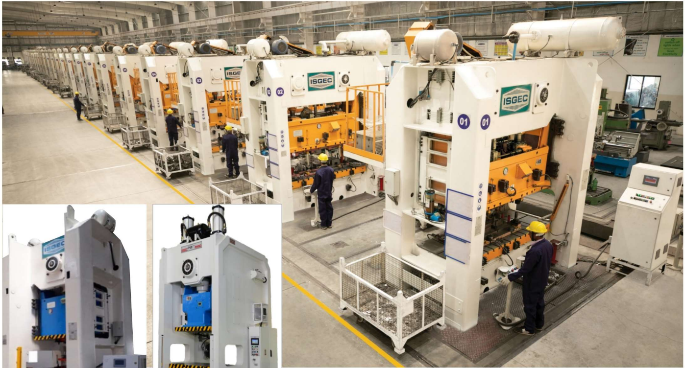
Battery of MAX 2 Series Monolithic Frame Double Crank Presses ranging from 200 T to 400 T capacity supplied for Progressive & Stamping Applications for Two Wheeler Components to Auto Tier-1 in India. MAX 2 Models are available from 200 T to 630 T
