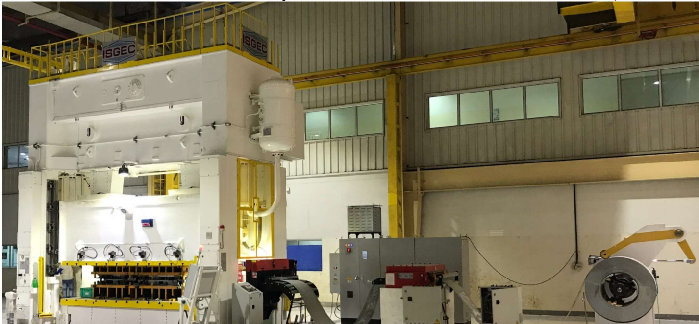
300 T Progressive Die Mechanical Press with Bed Size 4000 mm x 1500 mm, installed at Japanese OEM in India
