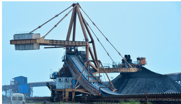
Stacker cum Bucket Wheel Reclaimer with stacking capacity of 6050 TPH, reclaiming capacity of 4500 TPH and boom length of 50 m.
