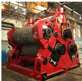
45\"X 90\" size mill-Casting, Machining and Assembly done at Isgec workshop.
