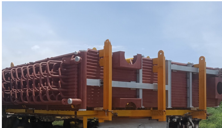
Superheater Assembly for waste-to-energy.
