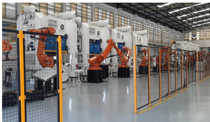
Robotic automation for Standard Mechanical Press.
