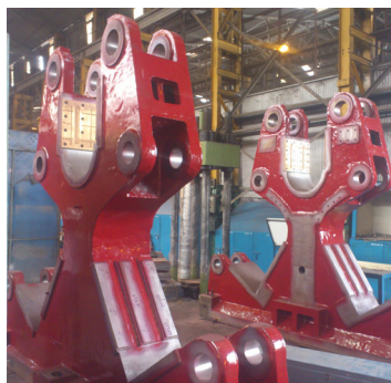
45\"X 90\" size mill-Casting, Machining and Assembly done at Isgec workshop.
