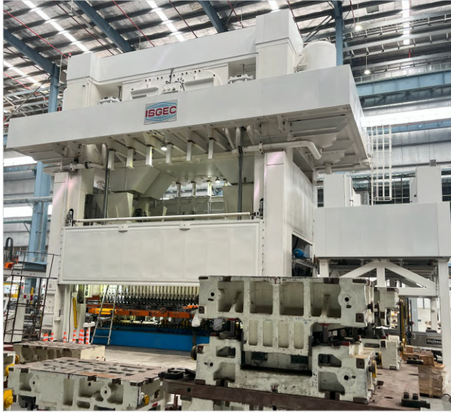
3000T Mechanical Transfer Press Line with a 60:40 loading pattern equipped with High Speed 3-Axis Servo Electronic Transfer System supplied to a major Automotive Tier-1 in India.
