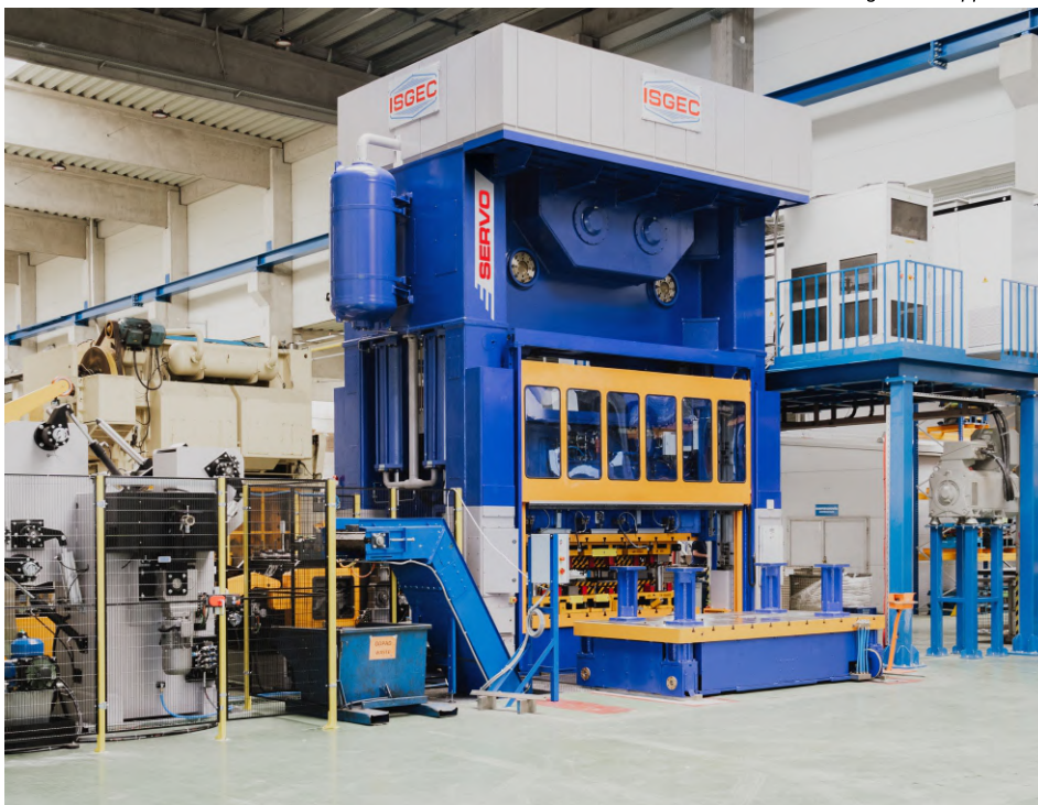
630 T Servo Mechanical Press with Bolster Size 3400 mm x 1600 mm and 3-50 spm installed in Slovakia for Progressive Application
