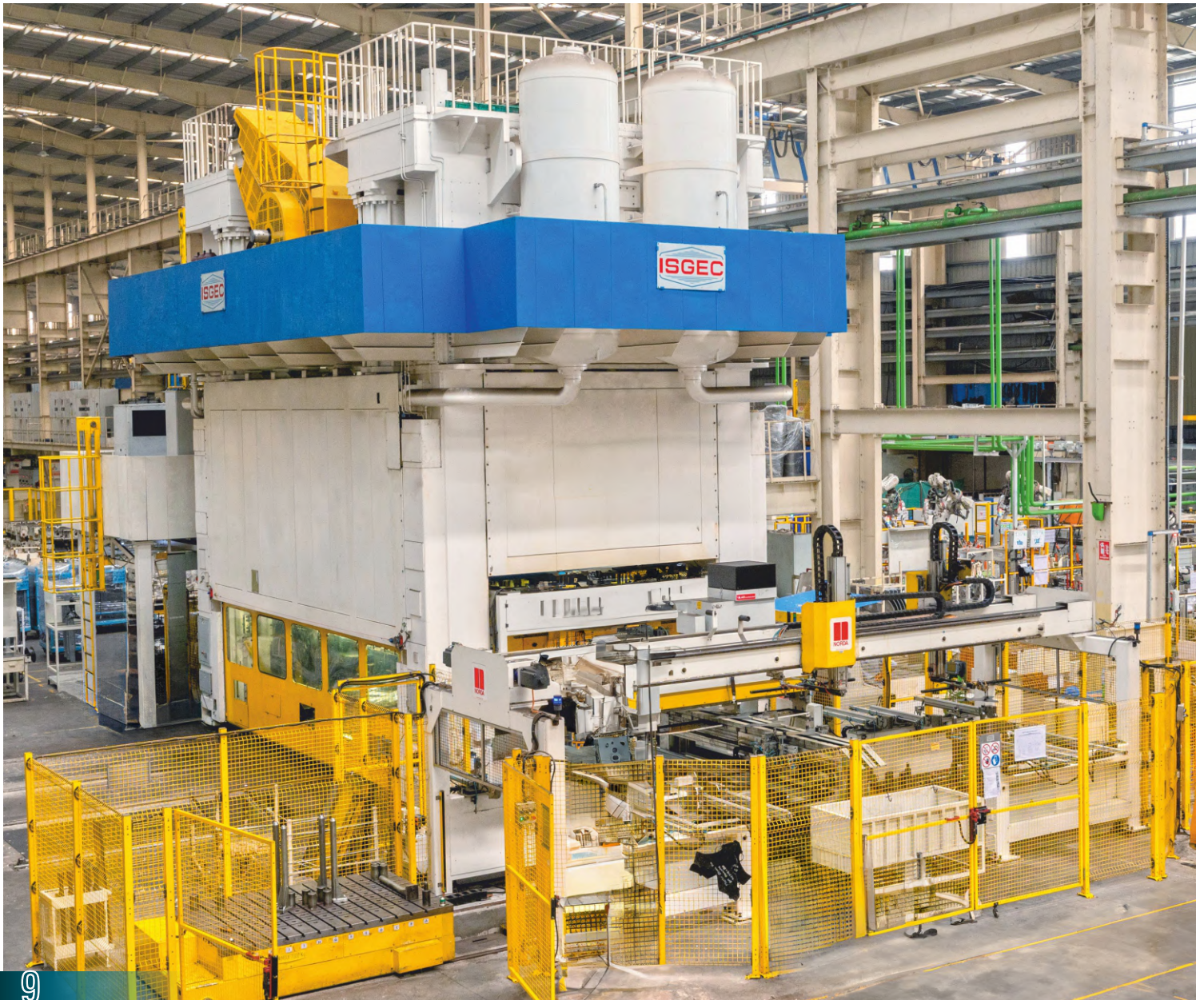
2500 T Link Drive Transfer Press (Bolster Size 6100 x 2500 mm) installed with a Tier-1 stamping supplier to Japanese OEM
