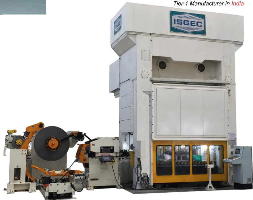
400 T Progressive Die Mechanical Press with Bed Size 4000 mm x 1500 mm, installed at Japanese OEM in India
